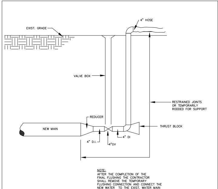
AFTER THE COMPLETION OF THE FINAL FLUSHING THE CONTRACTOR SHALL REMOVE THE TEMPORARY FLUSHING CONNECTION AND CONNECT THE NEW WATER TO THE EXIST. WATER MAIN ALL PIPING AND FITTING SHALL BE DISINFECTED TO THE SATISFACTION OF THE KCWA.
